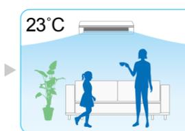
During cooling operation, with settings of 23°C for the room temperature and 30°C for Home Leave Operation.
