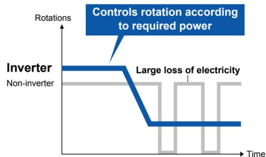
Inverter systems can cut energy consumption compared to non-inverter models. This helps to reduce household power bills and also lowers CO<sub>2</sub> emissions caused by electricity generation.
