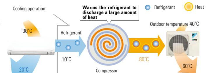
To discharge a large amount of heat outdoors, the refrigerant temperature must be higher than the outdoor temperature of 40°C. In this case, the temperature of the refrigerant returned from the indoor unit is 10°C. The refrigerant is heated to 80°C so the heat can be discharged easily.
