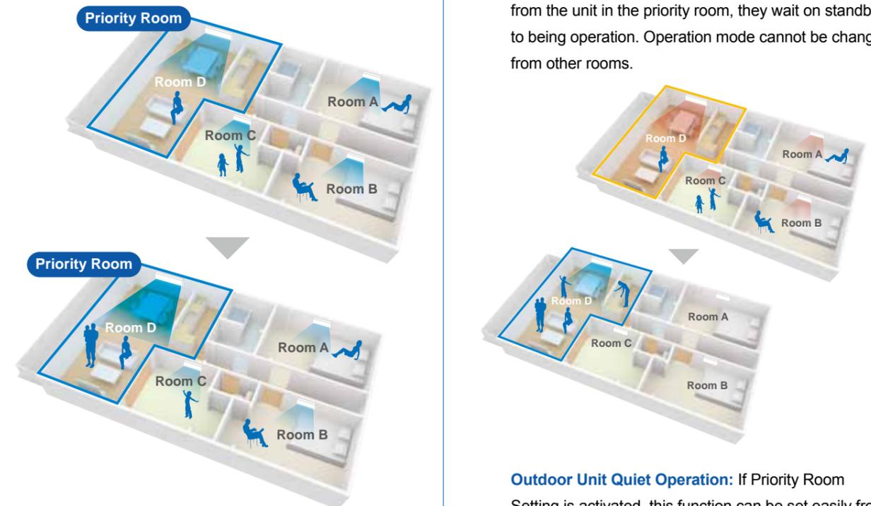
**Outdoor Unit Quiet Operation:** If Priority Room Setting is activated, this function can be set easily from the remote controller in the priority room.<sup>1,2</sup>
