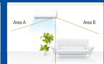
If no one is detected in either area A or B for 20 minutes, Intelligent Eye automatically adjusts the set temperature by approximately 2°C.
