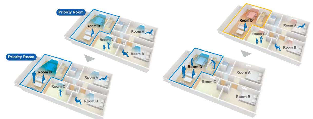
**Outdoor Unit Quiet Operation:** Outdoor unit operating sound pressure levels can be decreased from the rated operation sound using the wireless remote controller. If Priority Room Setting is activated during installation, this function can easily be set from the remote controller in the priority room<sup>1</sup>.
