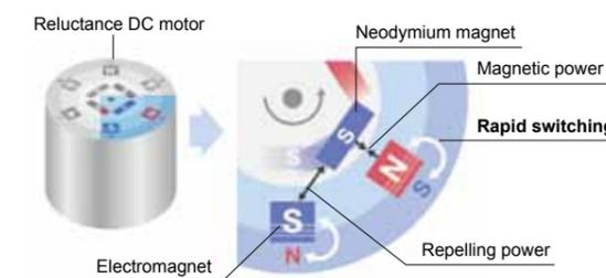
Embedding high-strength neodymium magnets in the shaft turns the entire centre of the motor into a powerful magnet. By rapidly switching the poles of this electromagnet, the Reluctance DC motor is able to produce even greater speed and power.
